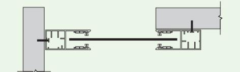
Undersize Fix (where some of the guide track will be into the opening)
