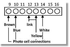
The black wire is not used and can be either cut out or just left un-connected.
